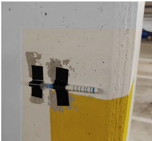
Figure 5: A Dosi-tube secured to a column.
