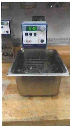
Figure 1: Warming up a sous vide water bath with PolyScience immersion circulator
