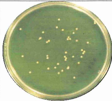
Figure 2: Heterotrophic Plate Count (Leboffe & Pierce, 1999). Live heterotrophic bacteria form clusters enabling the researcher to count the total number present.
