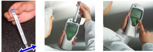
Figure 4. Luminometer and measurement of relative light units
